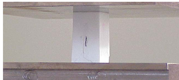
Fig.1. Compressive fracture behavior of syntactic foam.
