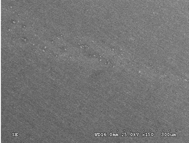
Figure 2- FSW 2219 and AA 2195 with highly dispersed precipitates exhibiting expected mechanical properties.
