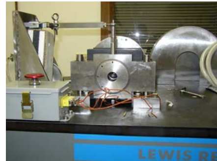
Figure 2: Lewis LRI-8H Bushing Tester
